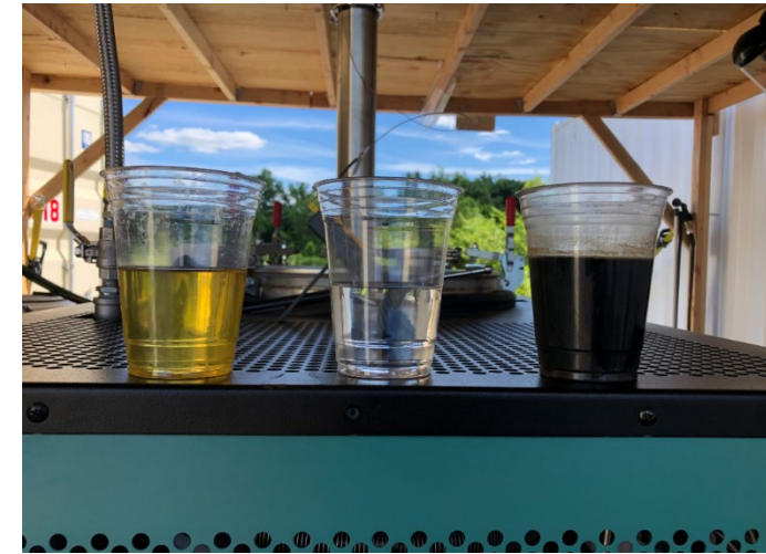
Picture of before and after of resin regeneration showing solution after regeneration (left), solution after distillation process (center), and concentrated still bottoms produced (right) after distillation for treatment via Plasma OR other ESTCP/SERDP technologies.
